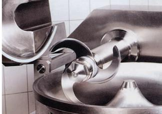
Three sickle-knives (as option) are used in order to cut and mix raw sausage products cleanly and fast. Meat and fat particles are evenly mixed. The finished raw sausage has a clear and high contrast cut pattern.
