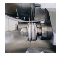
Due to the large distance between the knife head and the knife shaft bearing arm the cleaning of this area is considerably easier.
