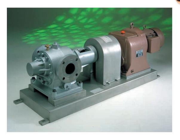
The Baynflax Cambridge Range of Chocolate Pumps can be used either in unit machines, such as Enrobers, for transfer pumping between unit machines and storage vessels, or for large volume applications such as bulk tanker unloading. When used with Fondant the pumps are supplied with hardened internal parts and vanes in order to suit the abrasive nature of Fondant.
